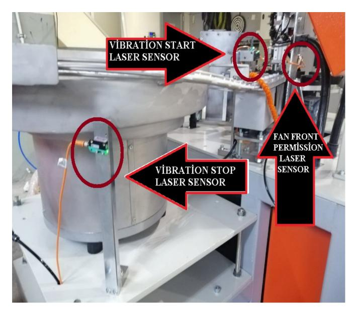
Fan Transport Front Permission Laser Sensor: This Sensor, if it detect fan, its let the fan move the front.
