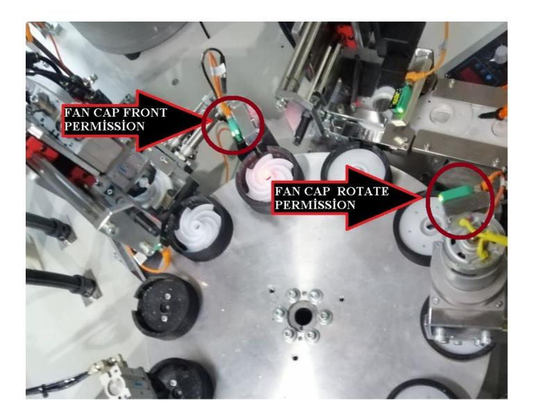
Fan Cap Work Permission Laser Sensor: This Sensor, if it detect fan, its let the fan cap operate.
