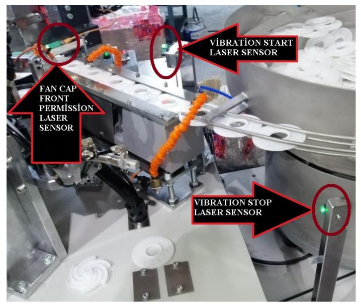
Fan Cap Front Permission Laser Sensor: This Sensor, if it detect cap, its let the fan cap move the front.
