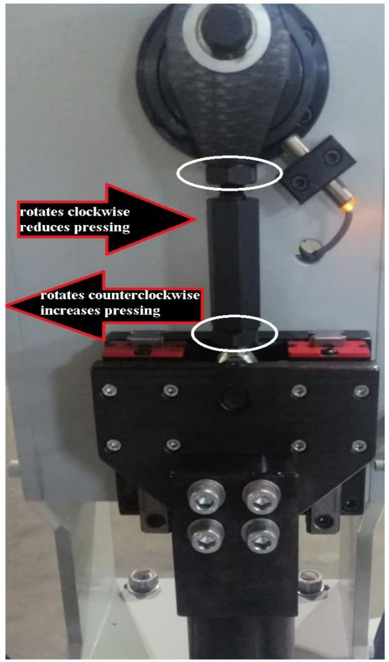
Firstly, unloose the upper and lower nut. Then left or right middle shaft rotate.
